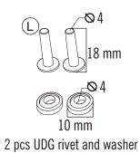
1 set package spare part UDG Frame Trolley + 2 pcs rivet and washer
